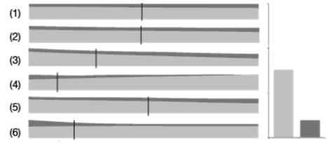
Figure 1. The output of the model shows the current selected parameters with their specific performance graph and the calculated heating (light grey) and cooling (dark grey) demands. It also displays how the parameters have to be changed to obtain a more effective solution.
